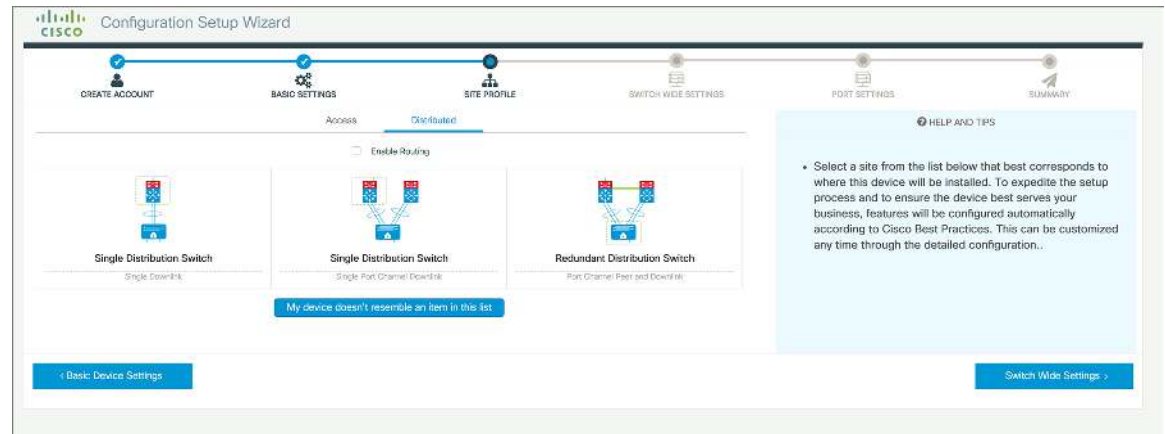
Figure 63: Site Profile - Distribution Switches (with Routed Access)
