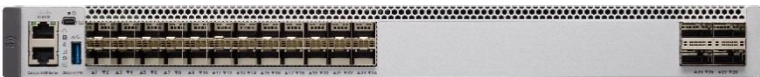
Figure 4. C9500-24Y4C: Cisco Catalyst 9500 Series high-performance switch with 24x 1/10/25G Gigabit Ethernet + 4x 40/100G Uplink
