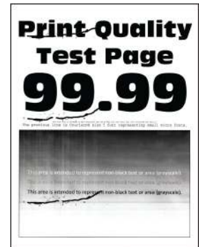
“Repeating defects” on page 264
