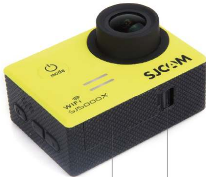
Battery door Battery door key
