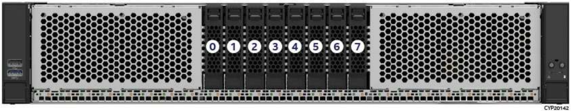
Figure 24. 2U 8 x 2.5" Front Drive Bay Configuration – M50CYP2UR208
