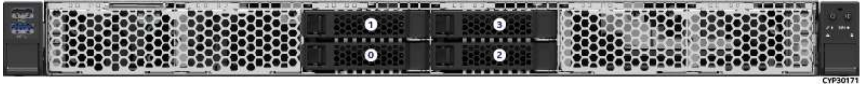
Figure 22. 4 x 2.5" Front Drive Bay Configuration – M50CYP1UR204
