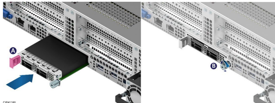
Figure 32. OCP* Module with Pull tab Installation (2U System Shown)
