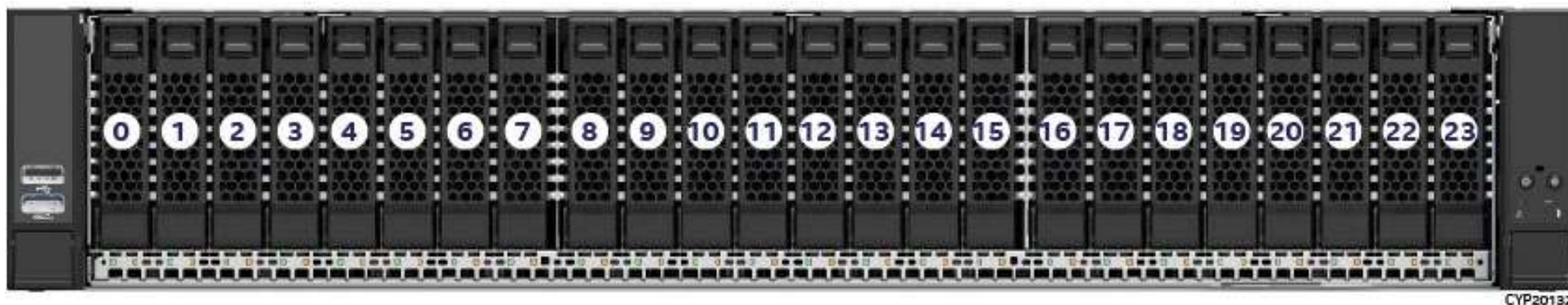
Figure 27. 2U 24 x 2.5" M50CYP2UR208 Front Drive Bay Configuration
