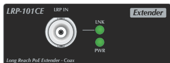
Figure 2-3: LRP-101CE Front Panel
