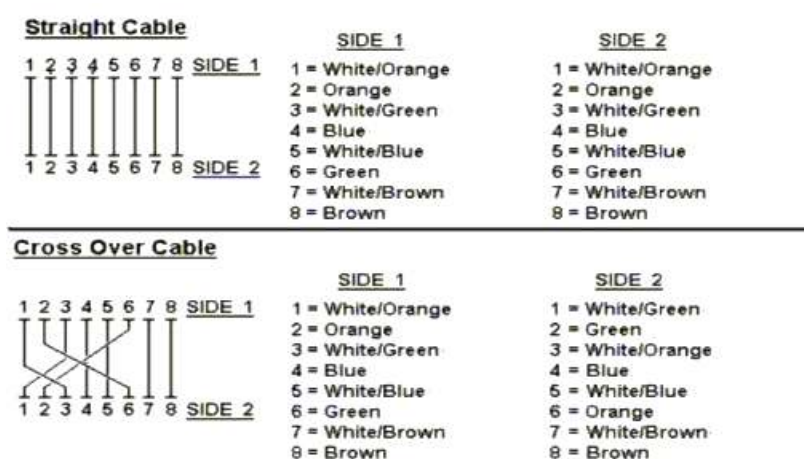
Figure A-1: Straight-Through and Crossover Cable
