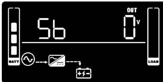
Figure 21: Display in standby mode
