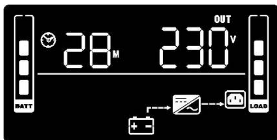
Figure 20: Battery mode display
